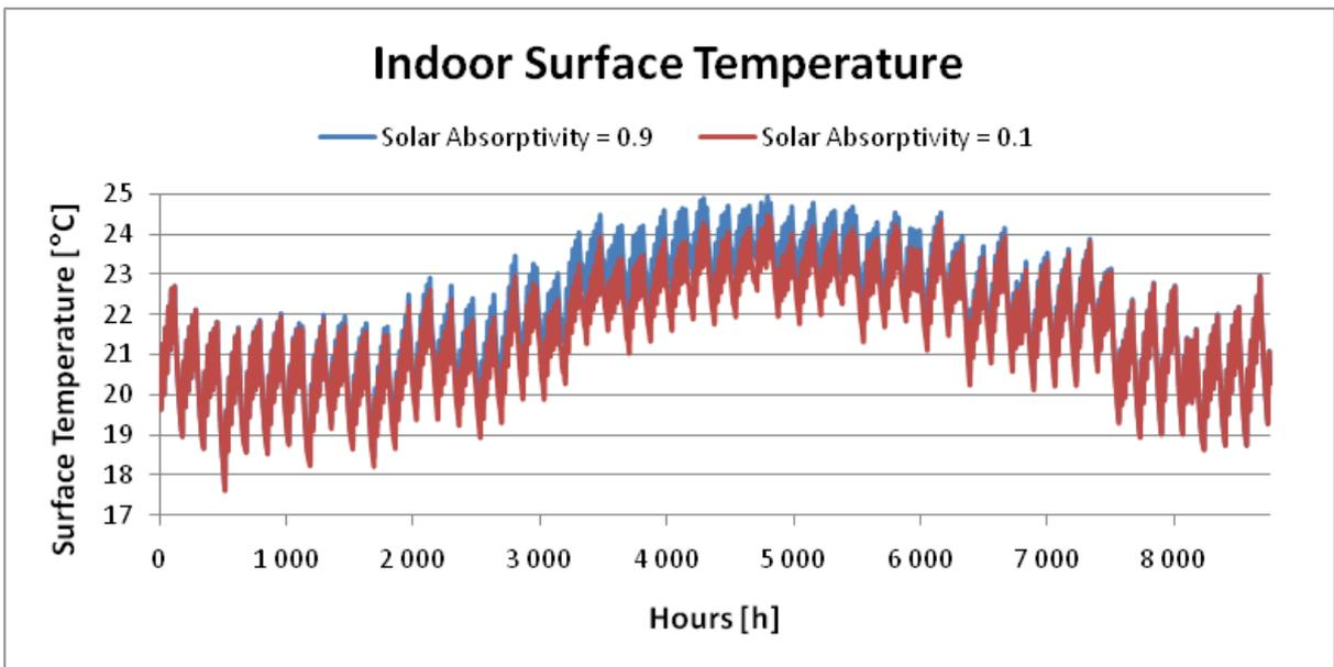
FIG 5. Indoor surface temperature with solar absorptivity = 0.9 and 0.1 (TRNSYS)
