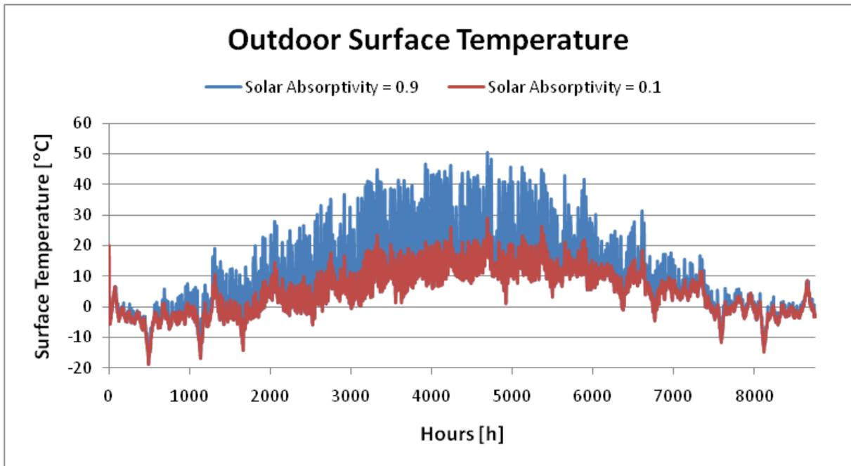
FIG 6. Outdoor surface temperature with solar absorptivity = 0.9 and 0.1 (TRNSYS)
