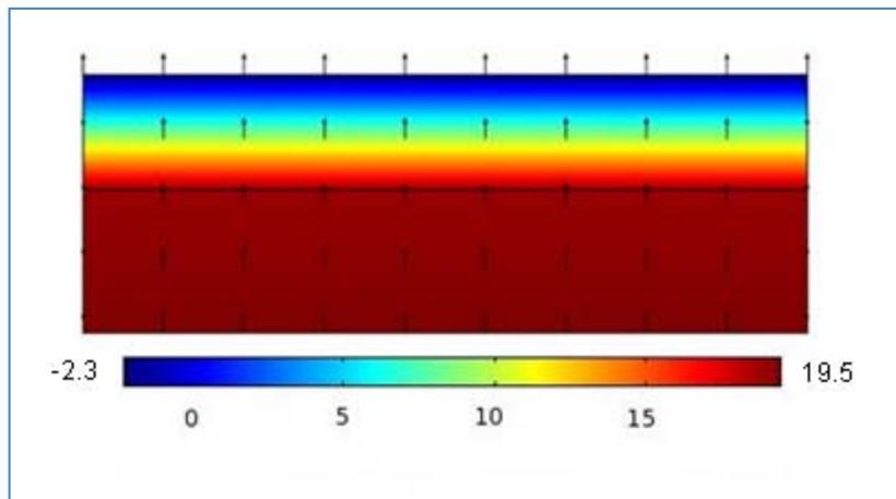
FIG 2. Steady state temperature distribution through the compact roof with -2.5 °C outdoors and 20 °C indoors. The heat flux is represented by arrows.
