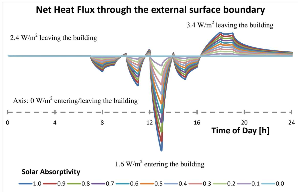
*FIG 3. Average heat flux through external surface boundary for 15<sup>th</sup> March transient simulation through varying solar absorptivities. Constant outdoor and indoor air temperatures. Solar data with weather fluxuations extracted from TRNSYS.*
