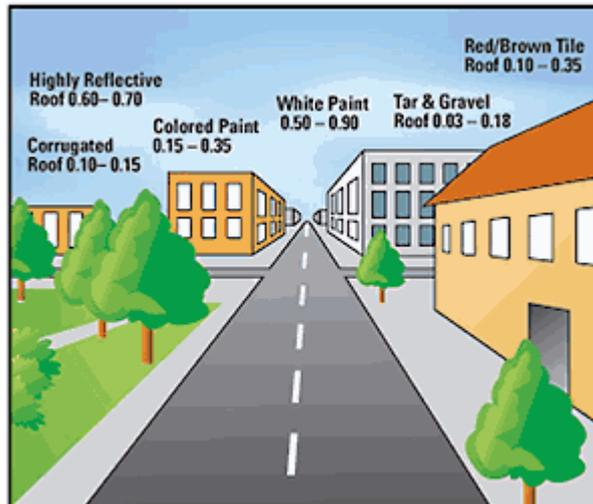
FIG 1. Illustration of possible reflection factors for various building components (Coolroofs, 2009)
