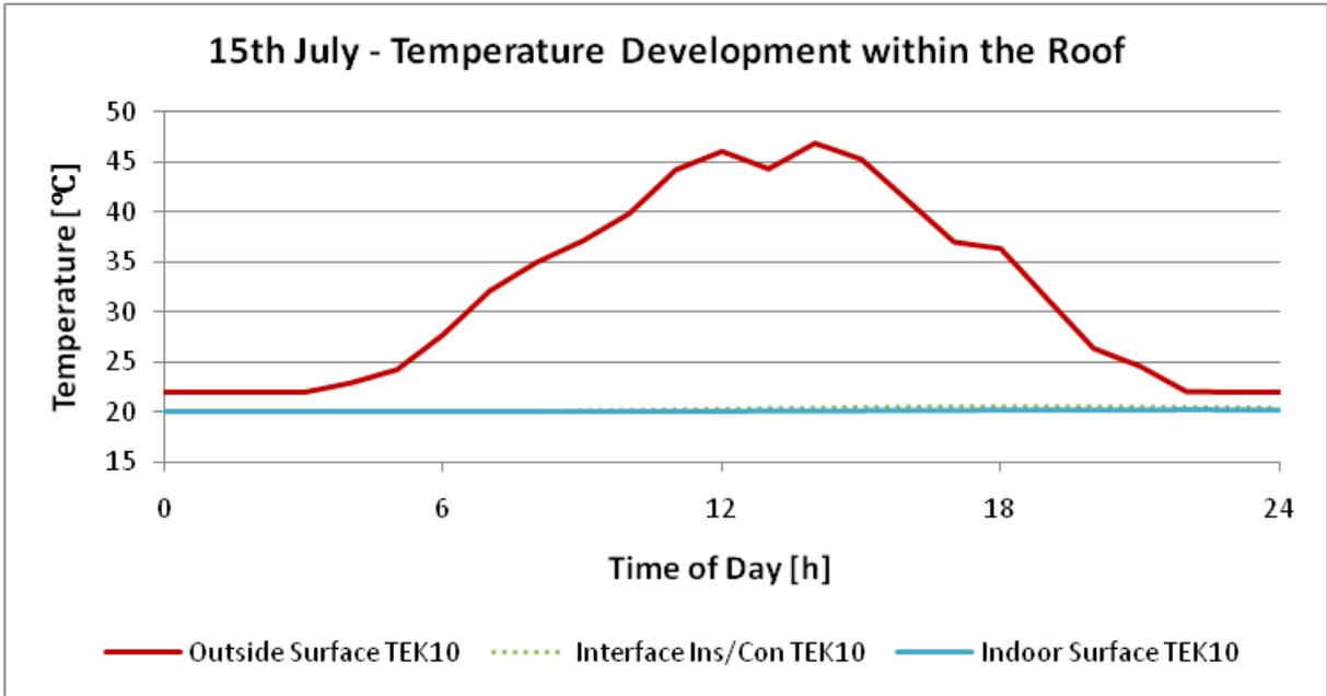
FIG 4. Temperature development of the indoor surface, interface between the concrete and insulation, and outdoor surface during 24 hours using solar data extracted from TRNSYS for the 15<sup>th</sup> July in Trondheim
